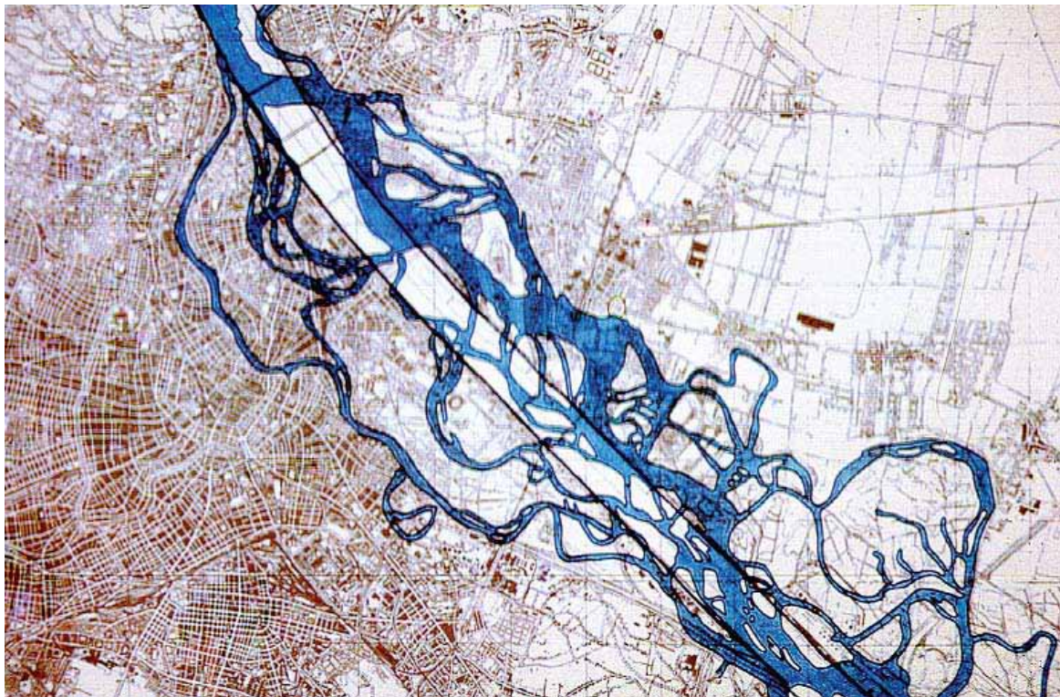
■ Figure 3. The Danube regulation at Vienna. The figure shows the braided network of channels and the engineered channel. The river regulation started in 1875.
